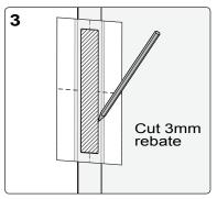
Remove middle section of end pull template and mark rebate outline on end of door. Use midline as height reference. Cut 3mm rebate.
